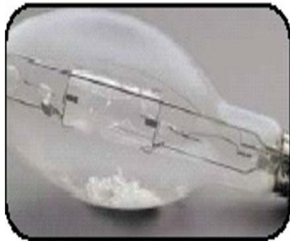
Ruptured arc tube contained in the in-tact outer jacket of an "O" rated lamp
